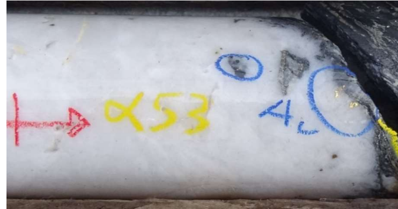
Visible gold in diamond hole FKH008 0.950m @ 40.5 g/t Au including 0.06m @ 786.1 g/t Au
